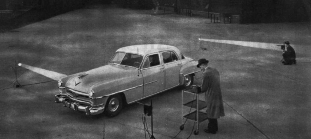
**GETAWAY TIMED BY ELECTRIC EYE.** This Chrysler breaks light beams at start and finish of getaway test, while electronic machines measure time to a split second.
